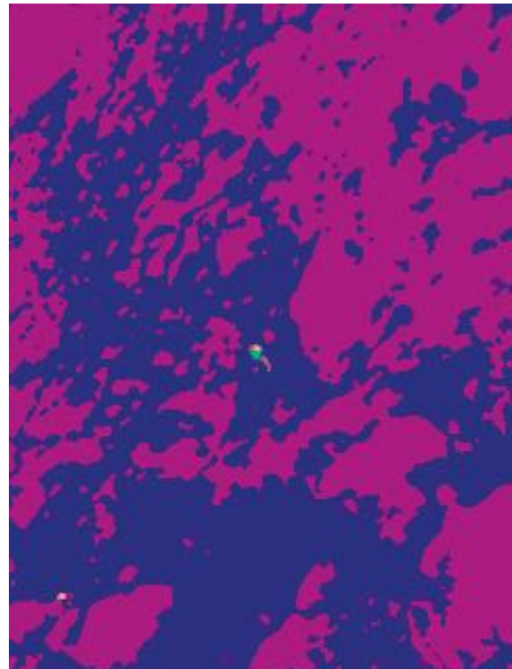
Fig 4. Segments of the image presented in Fig. 3. Segmentation is done using H and S component of the image (for presentation in this figure, V = 0.5 ).
